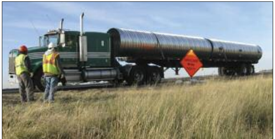
AUI sliplined 44-inch HOBAS Flush Relign pipe at Kirtland AFB.
